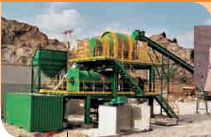
Complete mixing unit for the cleaning up of contaminated soil
